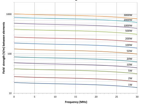
Field strengths shown are typical for free space. Proximity to conductive surfaces and the presence of the device under test will influence actual levels.
